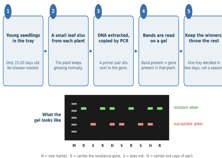
Fig. 4: The complete process from a seedling tray to a selection decision in about two days.
